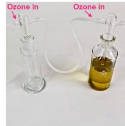
When you connect trap and oil bubbler make sure that you connect the ozone outlet of the trap with the inlet of the oil bubbler.
