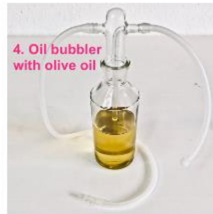
An oil bubbler is another gas washing bottle. The oil bubbler is where you pour olive oil in to ozonate it.
