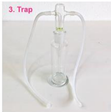
A trap is made of glass, it has an inlet which is connected to a stem, and an outlet. It protects the ozone generator from back-flowing oil.
